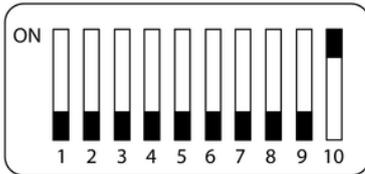
When DIP switch 10 is set to 'ON', the device operates in DMX mode and can be controlled by a DMX controller.
