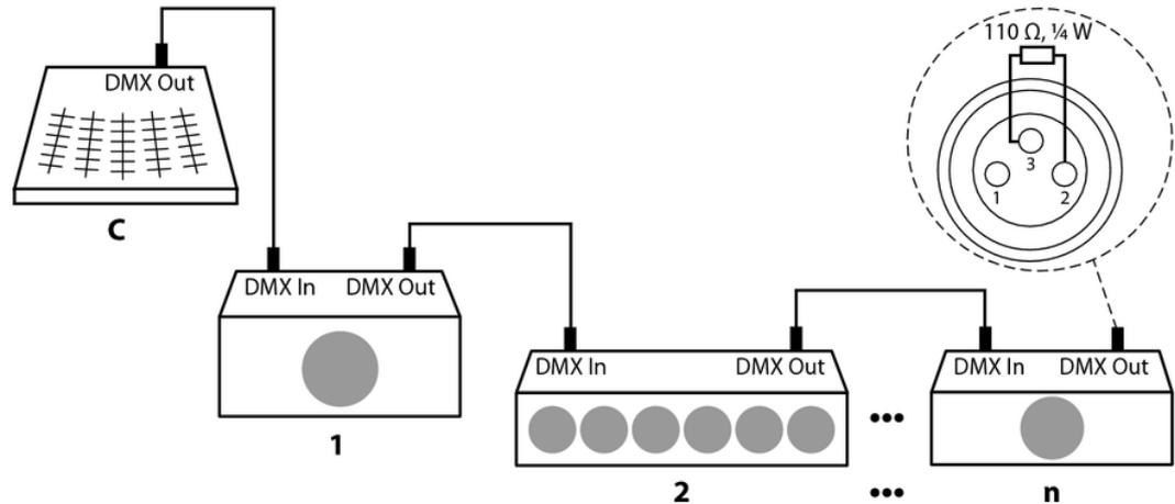
The flashing 'DMX' LED indicates an incoming DMX signal.
