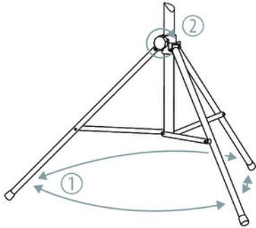
1. ➤ Unfold the feet of the tripods until the cross braces are in a horizontal position.
