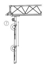
**6.** Loosen the two screws on the extension tubes. Pull out the extension tubes of the two stands to the desired height and fix both with the help of the locking screw on the stand.
