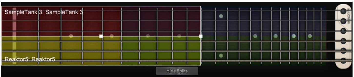
figure 20 - Here the Split 1/Split 2 and Split 3/Split 4 zones overlap. Notes played between the fifth and tenth frets trigger notes from two Split channels.
