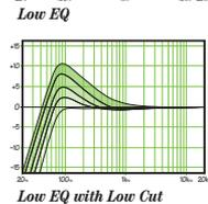
Used in conjunction with the low cut [5] switch, you can boost the low EQ without injecting a ton of subsonic debris into the mix.
