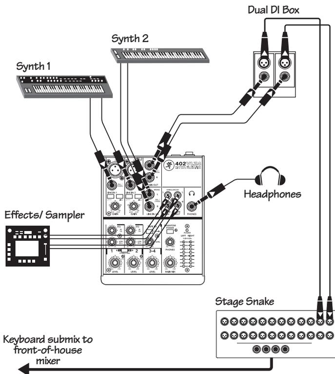
This diagram shows the stereo outputs of a synth connected to the line inputs of channels 1 and 2. The stereo pan switch is pressed in, so channel 1 only goes to the left of the main mix, and channel 2 only goes to the right.
