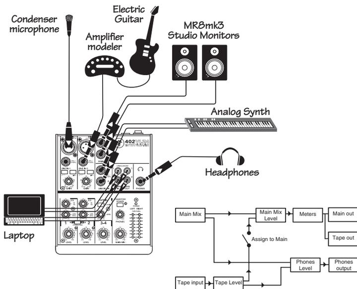
*This diagram shows a condenser microphone connected to channel 1's mic input, with the phantom power switch pressed in.*
