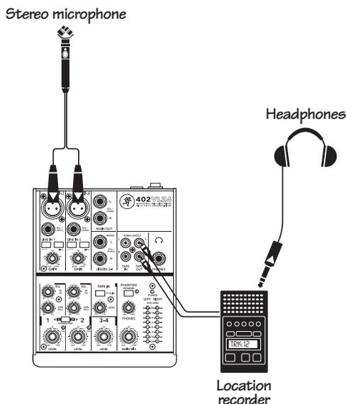
*This diagram shows the outputs of a stereo microphone connected to the mic inputs of channels 1 and 2. The stereo pan switch is pressed in, so channel 1 goes only to the left of the main mix, and channel 2 goes to the right.*
