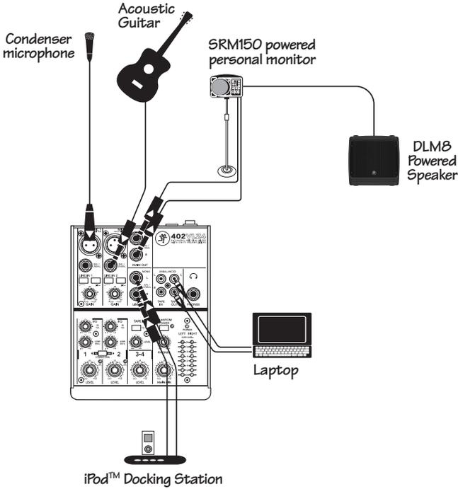
This diagram shows a microphone connected to channel 1's mic input, with the phantom power switch pressed in. A guitar is attached to the instrument input of channel 2, with the instrument switch pressed in.
