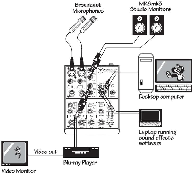
*This diagram shows two voice-over microphones connected to the mic inputs of channels 1 and 2.*
