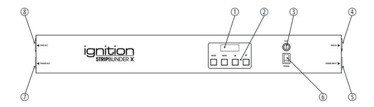
1 Display 2 Function and control buttons [MENU]: opens the main menu. Arrow button ▲: increases the displayed value by one. Arrow button ▼: decreases the displayed value by one. [MODE]: selects an operating mode. 3 Fuse holder. Should the fuse have blown, disconnect the unit from the power supply and replace the fuse with a new fuse of the same type. 4 [DMX IN] DMX input. 5 [POWER INPUT] Lockable Power Twist input socket for power supply. 6 Main switch. Switches the device on and off.
