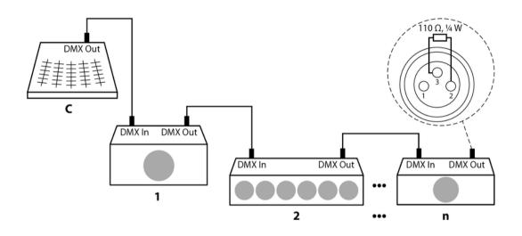
If the cable length exceeds 300 m (328 yds.) or the number of devices is greater than 32, the signal must be amplified using a DMX booster.
