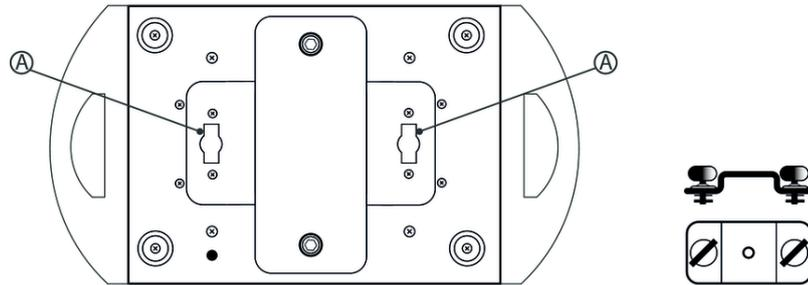
A Quick lock openings for Omega brackets
