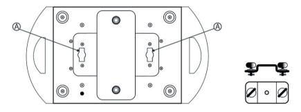
A Mounting points for 1/4-turn fasteners used for omega brackets
