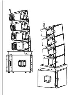
1) Fix the HDL fly bar on subs as shown in the picture.
