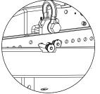
8 Check that all the pins are secured and locked.
