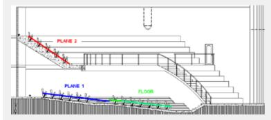
Enter the height, length and elevation of up to three planes.
