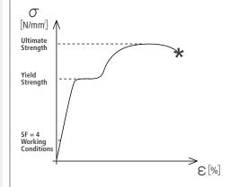
The safety factor is the result of the forces acting on fly bar's and system's front and rear links and pins and depends on many variables:
