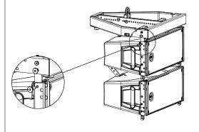
4) Reverse and connect the 2 rear bracket to the fly-bar using 2 quick lock pins. The first HDL has to be fixed always starting at 0° with respect of the frame. No other angles are allowded.
