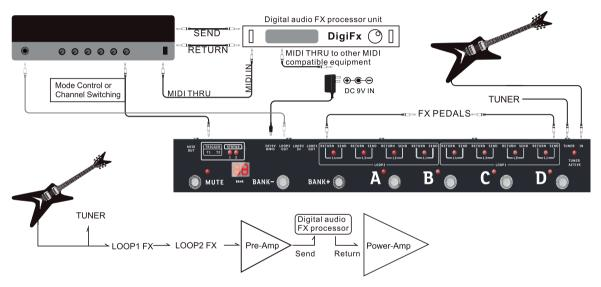
If your instrument is connected to the input [IN] and your amplifier to the output [LOOP2 OUT], eight effects processors can be looped into the signal path. In this example, an audio processor arranged behind the preamp in the signal path is controlled by a third device.
