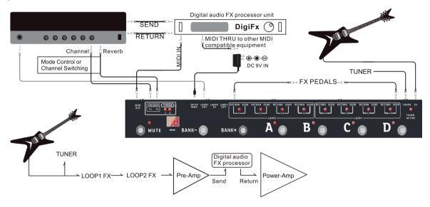
If your instrument is connected to the input [IN] and your amplifier to the output [LOOP2 OUT], eight effects processors can be looped into the signal path. In this example, the MIDI output controls an audio processor that is arranged behind the preamp in the signal path.
