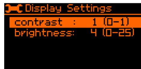
Press the Up/Down buttons to adjust the value of the highlighted setting
