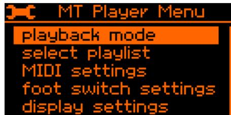
Use the Next / Previous buttons, or alternatively the Up / Down buttons, to navigate to the desired menu setting, which will be highlighted on the display.
