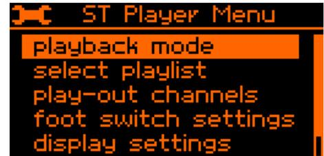
Use the Next / Previous buttons, or alternatively the Up / Down buttons, to navigate to the desired menu setting, which will be highlighted on the display.
