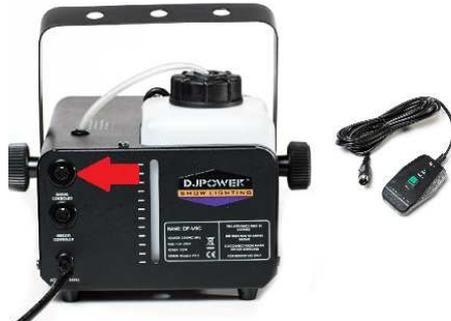
3. The machine needs 4,5min to heat up. Now you can push the green Fog button on the control and the machine starts. The button is momentary, which means that the fog machine will only output while button is pressed.
