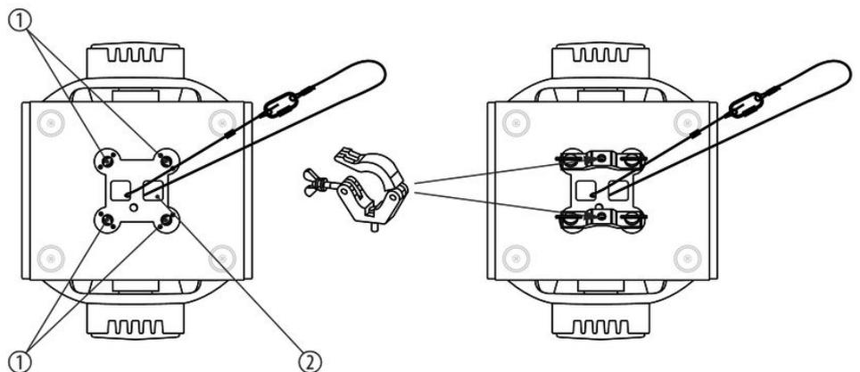
1 Quick lock openings for Omega brackets
