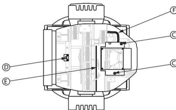
5. ➤ Loosen the two Phillips screws holding the illuminant cover (marked in the illustration by 'C') and remove the illuminant cover.
