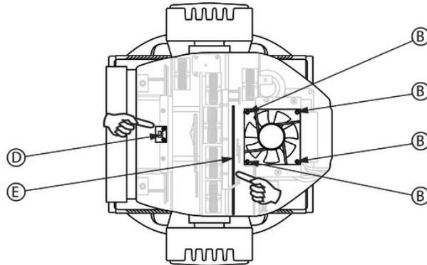
4. ➤ Check that you have removed the proper cover. Compare the exposed interior of the unit with the illustration. If you can see the heat sensor (marked in the illustration by 'D') at this point, the proper side of the case has been opened. If the correct side of the case is open, you can also clearly see the colour wheel (in the figure marked by 'E').
