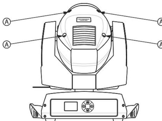
10. ➤ Put the upper part of the housing back on the base. At that point, both housing parts must engage in the circumferential seal profile. Replace the four Phillips screws ('A') to the top of the housing and tighten them.
