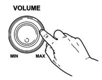
Adjust the rotary control [VOLUME] for a pleasant volume for playback and practising. Turn this control clockwise to increase the volume. Turn it counter-clockwise to reduce the volume.
