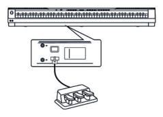
You can connect a triple-pedal (Sustain, Sostenuto and Soft) to the digital piano via the connection socket on the bottom of the unit.
