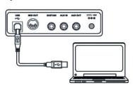
You can connect the digital piano to exchange data with a PC via the USB port.
