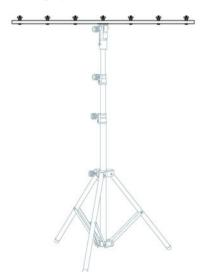
Mount the TV spigot (28 mm adapter) to the tripod and tighten it with the locking screw at the mounting; put on the truss beam and fix it in the desired position with the wing nut. Affix up to six spotlights to the truss beam. Spread the spotlights evenly on the truss beam. Observe the instructions of the respective manufacturers. The maximum load capacity of 45 kg in total must not be exceeded.
