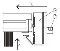
Slide the mounting clamps (5) for the railings (4) into the profiles of the respective stage platforms. As shown in the following figure, the guiding stub of the mounting bracket in the profile must be aligned upwards.
