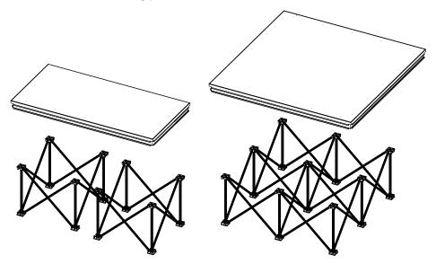
Unfold the feet completely and place them on an absolutely flat, solid and sufficiently stable ground. Put the stage platforms so on the feet, that the tops of the feet are respectively located at the corners of the stage platforms. The stage platforms must snap in on all feet.
