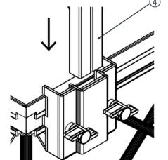
Insert the railings (4) from the top all the way into the mounting brackets.
