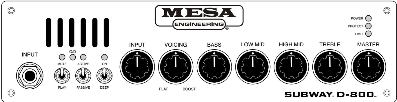
**INPUT JACK** This jack is the instrument INPUT that feeds the first stage monolithic J-FET buffer amp of the SUBWAY D-800. The input sensitivity of this input buffer amp is adjustable with the ACTIVE/PASSIVE switch, the ACTIVE position being about 10dB less sensitive (lower gain) than the PASSIVE position.
