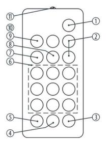
To use the remote control, point it with the infrared diode to the infrared sensor on the unit and press the desired buttons. The maximum distance from the unit is about 9 m. The device will only respond to the remote control signals if it is not controlled via DMX.
