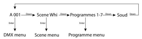
Press [DOWN] while 'A001' is flashing in the display to call the preprogrammed scene. Press repeatedly [DOWN] to call one of the 7 programmes. Press, if necessary repeatedly, [DOWN] to set the device to sound-to-light mode.
