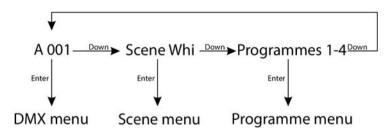
Press [DOWN] while 'A001' is flashing on the display to call up the preprogrammed scene. Press [DOWN] repeatedly to call up any of the 4 programmes.
