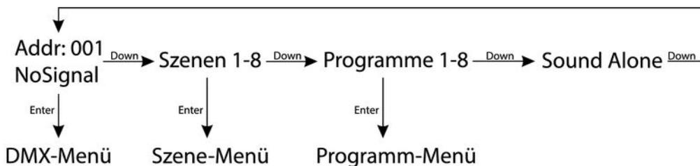
Press repeatedly *[DOWN]* while 'A001' is flashing in the display to call up one of 8 preprogrammed scenes, one of 8 programmes or to set the device to sound-controlled mode.
