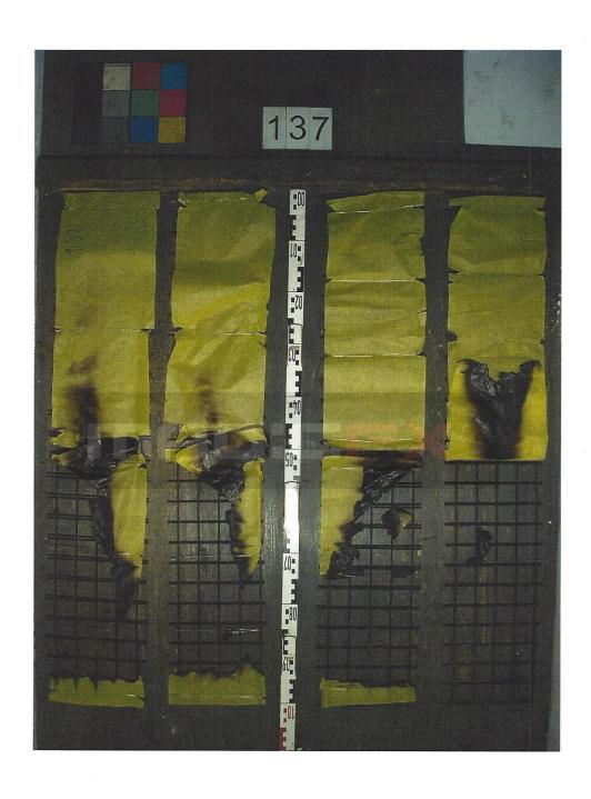
Picture 1: Appearance of specimen A after the test
