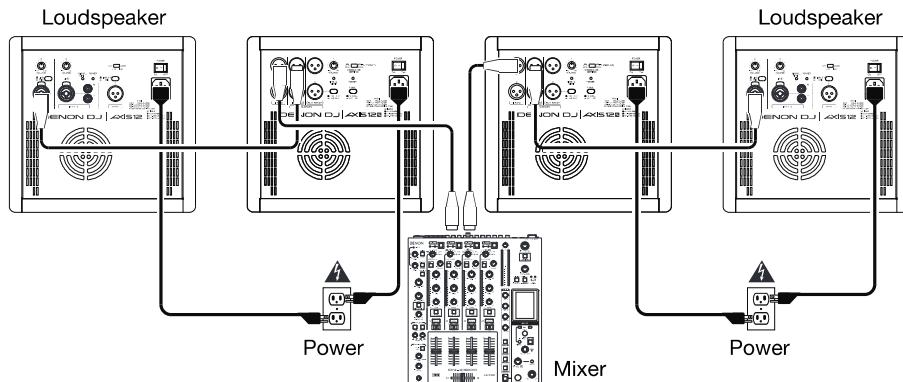
Using XLR cables, connect the left and right outputs of your mixer to **Input 1** of each subwoofer, and then connect **High-Pass Output 1** of each subwoofer to the input of each loudspeaker.
