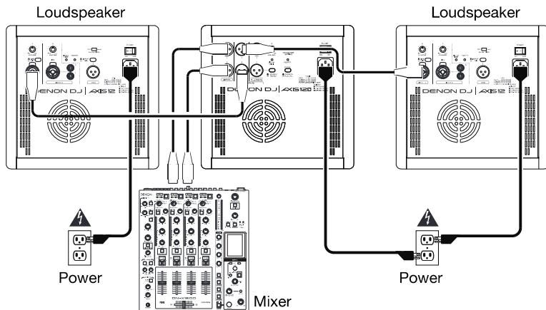
Using XLR cables, connect the left and right outputs of your mixer to the inputs of your subwoofer, and then connect the **High-Pass Outputs** of the subwoofer to the input of each loudspeaker.
