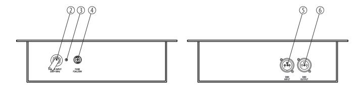
2 [POWER INPUT] | Mains cable for the power supply.
