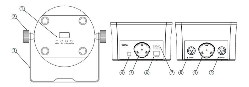
Display and function buttons. [MENU] Activates the main menu and toggles between menu items. Closes an opened submenu. [UP], [DOWN] Toggles between the menu items of a menu level, increases or decreases the displayed value by one. [ENTER] Selects an option of the respective operating mode, confirms the set value. 2 Locking screws for the mounting bracket. 3 Bracket for floor placement or hanging. 4 [POWER] Connection socket for the 15 V power supply unit. 5 Rechargeable battery compartment.
