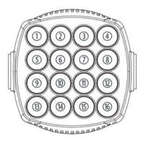
The adjacent figure shows the numbering of the individually controllable LEDs.
