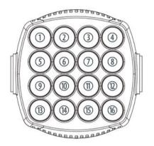
The adjacent figure shows the numbering of the individually controllable LEDs.
