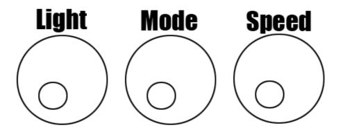
For manual operation there are, on the back of the device, 3 rotary controls.
