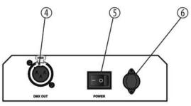
1 [1]...[6] Channel faders 1 through 6. Use the channel faders to individually control DMX channels 1 ... 6. 2 [POWER] Power indicator. 3 [MASTER] Master fader. The master fader serves as the sum controller for the six individual channels. 4 [DMX OUT] DMX output. 5 [ON/OFF] Main switch. Turns the device on and off. 6 Connection socket for the power adapter.
