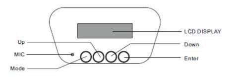
Press MODE to get to the menu. With UP/DOWN you can select the required point of menu. Confirm your selection with ENTER. With UP/DOWN you can make your settings after this confirm your settings with ENTER.
