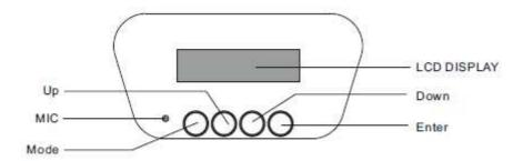
Press MODE to get to the menu. With UP/DOWN you can select the required point of menu. Confirm your selection with ENTER. With UP/DOWN you can make your settings after this confirm your settings with ENTER.
