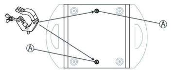
A Quick lock openings for Omega brackets
