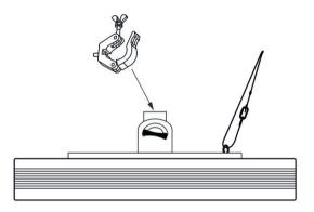
The mounting rails and fastening lugs are used for secure serial mounting of several Effect panels. Secure each individual device additionally with a safety cable, which is routed through the safety eyelet on the rear side, as shown in the following figure.
