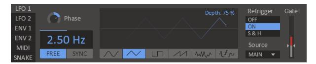
Multipass is equipped with two **low frequency oscillators**, or LFOs for short, which are ideal for modulating parameters in an oscillating and rhythmic fashion.
