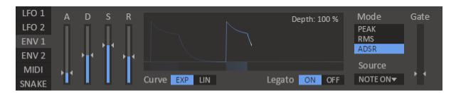
Multipass is equipped with two **envelopes**, which can be used to modulate parameters using the audio volume or MIDI note events.
