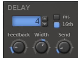
The **feedback** knob controls the decay rate of the echo. At the maximum value the effect will keep echoing forever. At the minimum value the echo will bounce just once. Values in between will result in a natural decaying echo.
