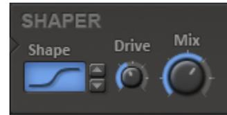
The first mode of shaping is **overdrive**. This performs a soft clamp on high amplitudes, resulting in a fairly sharp, aggressive distortion that can be used for making sounds with more edge.
