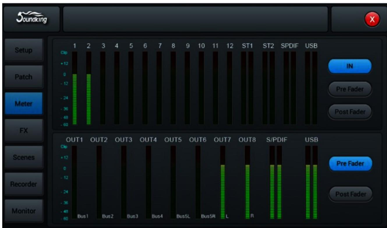
The input signals are processed in the IN, pre-fader and post-fader modes. Default setting: Pre-Fader. The selection is made using the three buttons to the right of the input displays.
