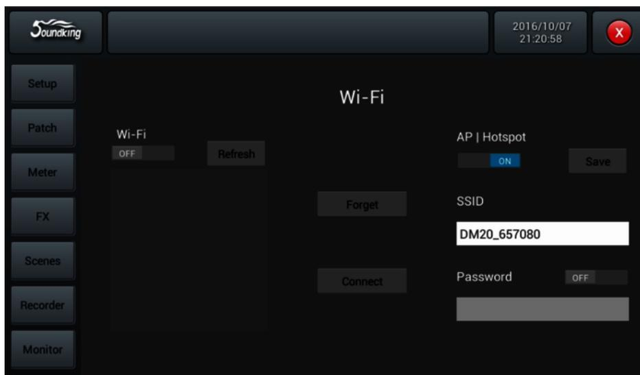
Deactivate the WiFi function [WiFi - OFF] and activate the AP function [AP-/Hotspot - ON]. Enter the standard AP name for the mixer under [SSID]. This name can be changed. Set a password if desired.
