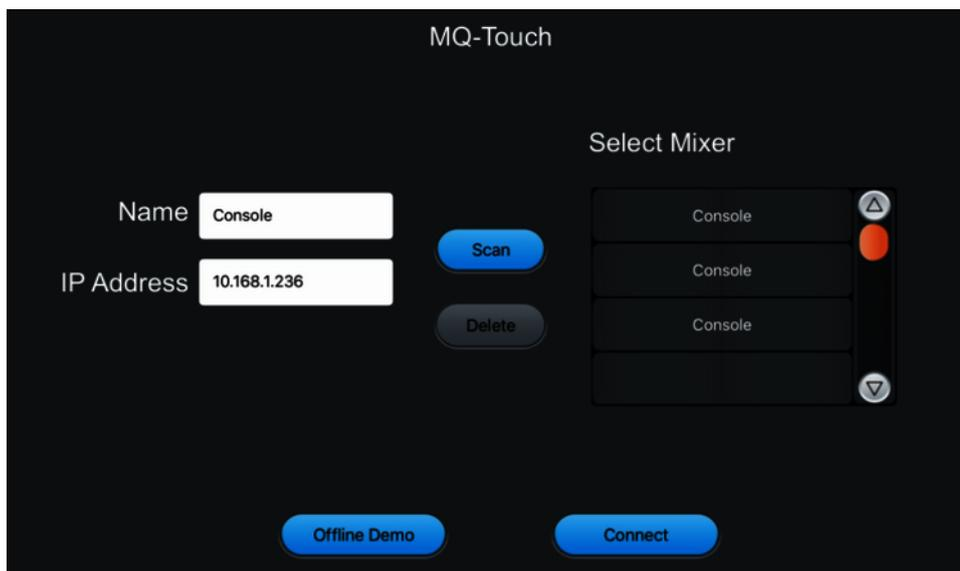
Enter the mixer name and the IP address manually or select the mixer from the list of found devices ([Scan]). Use [Connect] to establish the connection. Use [Delete] to delete a marked list entry.
