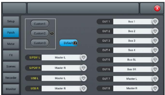
In this menu, the assignment of the channels to the available outputs can be adjusted.
