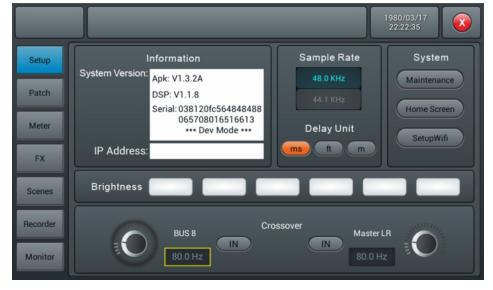
In this menu, the settings for WiFi operation can be set. Make sure the WiFi module is connected to the device, and then press [Setup] to open the menu. "Device Settings".
