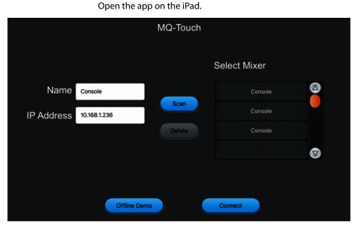
Enter the mixer name and the IP address manually or select the mixer from the list of found devices (*[Scan]*). Use *[Connect]* to establish the connection. Use *[Delete]* to delete a marked list entry.
