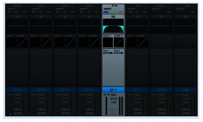
For the stereo inputs, the input, equalizer, dynamic, bus-send and output settings can be adjusted analogously to the microphone inputs.
