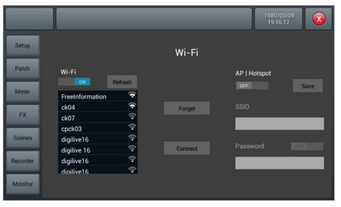
If necessary, activate the WiFi function [*WiFi - ON*] and tap the desired list entry to select a network. Press [*Connect*] to establish the connection. Use [*Refresh*] to perform a new search for networks, use [*Forget*] to delete the marked network from the list.
