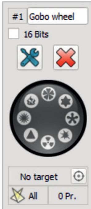
Get the instruction manual of your desired device ready and open the page with the DMX channels. If your device has multiple DMX modes, choose the channel mode that covers all the features you need. Now start recreating the functions in the profile editor step by step. To do this drag and drop the corresponding function into the lower area.
