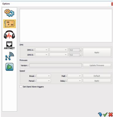
In this tab you have the possibility to adjust the settings for connected interfaces. All detected interfaces are listed first and identified by their serial number. Select the corresponding interface and then make the respective settings. Note: Only by clicking 'Apply' the settings are written to the interface.
