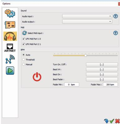
This section is for configuring the audio inputs and outputs. If you want to analyse audio signal from the same computer, you can loop it through internally. Depending on the operating system, different approaches are possible here.
