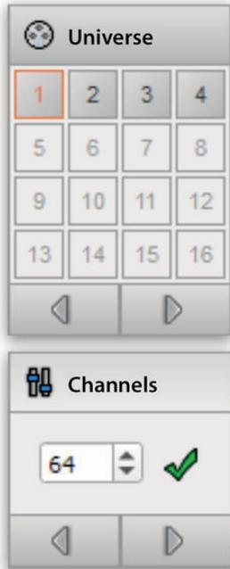
To test un-patched devices or to control DMX channels, you can select the 'Channels' tab. On the right side, select the universe in which you want to make changes.
