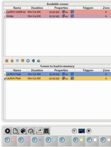
Each DMX Joker interface has a standalone feature to varying degrees. This means that scenes can be saved in the interface and can be played without a computer. All you have to do is power the interface with a USB power supply.
