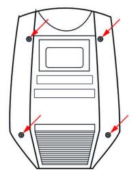
**9.** Close the housing with the two covers and secure them with four cross-head screws each.
