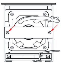
**3.** Remove the small metal plate on the back by unscrewing the two screws.
