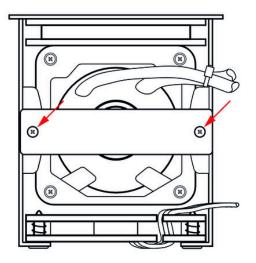
**8.** Fasten the small metal plate with the two screws on the back.
