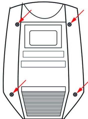
**9.** ➤ Close the housing with the two covers and secure them with four cross-head screws each.
