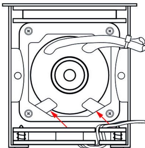
4. ➤ Align the head of the unit so that the metal brackets of the illuminant are aligned as shown in the figure.
