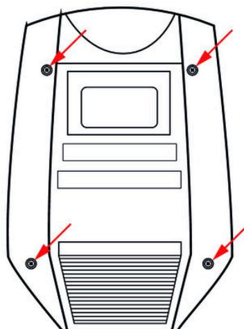
1. ➤ Remove one of the covers from the head of the unit. To do this, loosen the four cross-head screws using a suitable screwdriver. Then carefully remove the cover from the unit.
