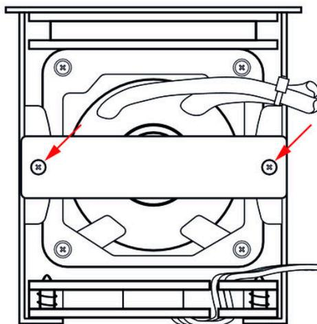
3. ➤ Remove the small metal plate on the back by unscrewing the two screws.
