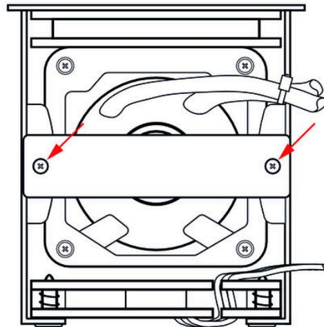
**8.** ➤ Fasten the small metal plate with the two screws on the back.
