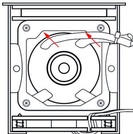
7. ➤ Re-insert the illuminant into the retainers. Be sure to keep the illuminant at the corners under the bracket.
