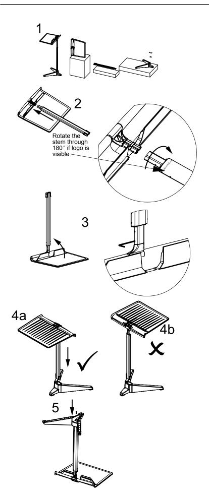
1. Check that you have all of the components required for your Alto stands. Stands supplied in 8 up packs are in 3 different boxes, one containing 8 tray assemblies, one containing 8 stem assemblies and one containing 8 base assemblies, 8 screws and 1 2.5mm hex key.
