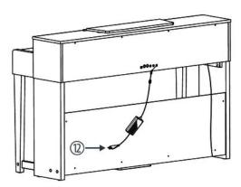
Insert the DIN plug of the pedal cable into the provided socket on the bottom side of the digital piano. Insert the plug into the corresponding socket on the bottom side of the digital piano. Fix the cables to the base frame and move the digital piano to the desired position.
