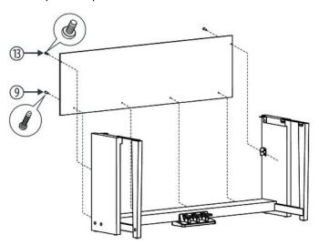
Fasten the back panel with four screws  $\times$  15BA at the Foot pedal unit with two screws M6  $\times$  12 at the washer of the side panels.
