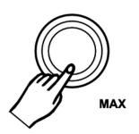
Adjust the rotary control [VOLUME] for a pleasant volume for playback and practising. Turn this control clockwise to increase the volume. Turn it counter-clockwise to reduce the volume.
