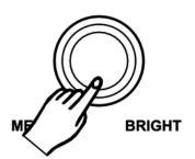
Use the rotary control [BRILLIANCE] to adjust the sound quality. Turn this control clockwise to produce a brighter sound. Turn it in the opposite direction to produce a darker sound with less presence.
