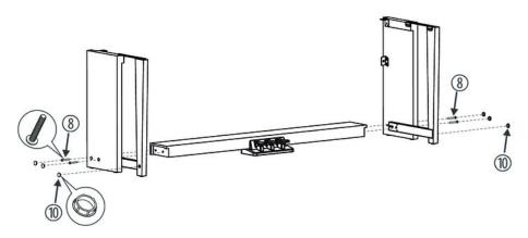
Put the pedal box between the left and right side panel and use two screws  $M6 \times 50$  on each side to affix both side panels to the pedal box.
