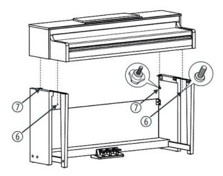
Place the digital piano case on the frame and secure it to the side panels with two screws M6  $\times$  18 and the two thumbscrews.
