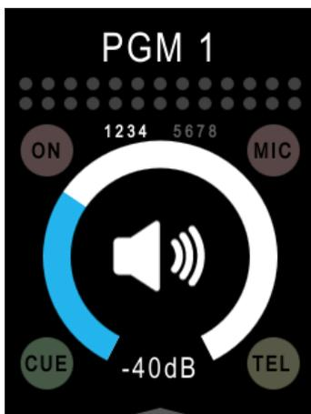
ON: At least one channel is turned on and the fader is opened
