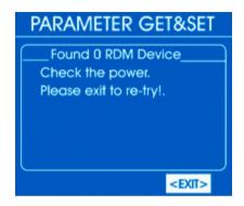
In this case, check the wiring and the correct fit of the connectors.
