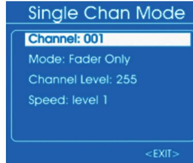
5. ➤ To select the channel on which the data should be sent, select the item *'Channel'*. Press the jog wheel. Use the jog wheel to set a value between 1 and 512 – or *'All'* for transmission on all channels.
