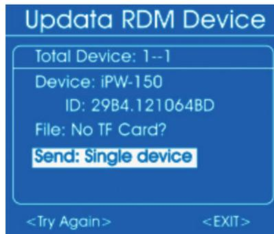
5. ▶ To retrieve a parameter, select it with the jog wheel and press the jog wheel. Select '*Single device*' (transmission to one device) or '*All devices*' (transmission to all devices) and press the jog wheel.
