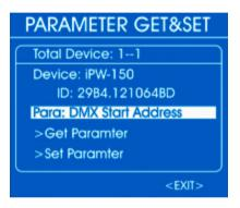
**4.** Use the jog wheel to select 'Para: DMX Start Address' and press the jog wheel.
