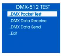
**3.** Select one of the submenus 'DMX Packet Test', 'DMX Data Receive' or 'DMX Data Send'.
