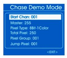
23. Use the jog wheel to select the setting to be changed and press the jog wheel. Turn the jog wheel to select or adjust a value. The following table shows the menu items and choices.
