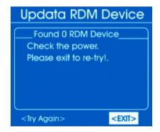
In this case, check the wiring and the correct fit of the connectors.
