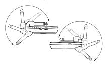
Plug the transmitter into the 1/4" phone socket of the instrument whose signal you want to transmit. The transmitter flashes five times. During transmission, the LED indicator lights up.
